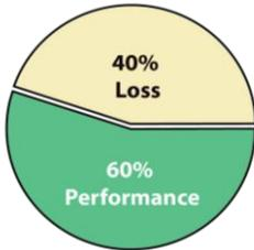
The graph shared a performance ratio between system delivered BTUs to the building space divided by equipment rated capacity in BTUs. A typical system only delivered about 60% of the equipment rated BTUs the equipment was capable of producing to the building space. Most utility programs didn't look at delivered performance. This airside approach test-in approach identified additional defects in the system delivery system in addition to addressing proper installation.
